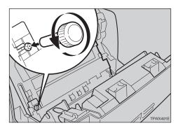
6 Holding the green inset grips of the photoconductor unit, pull the top of the unit forward.
